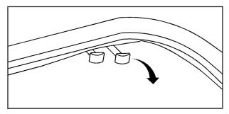
Open the trunk and pull one or both of the handles located on the upper part of the trunk opening. The driver's side handle will open the larger side of the seatback. The passenger's side handle will open the smaller side of the seatback. Notice: Folding a rear seat with the safety belts still fastened may cause damage to the seat or the safety belts. Always unbuckle the safety belts and return them to their normal stowed position before folding a rear seat.
